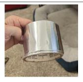
Silver tape used to cover all window weep holes before putting all coverings on. Leaves no residue.
